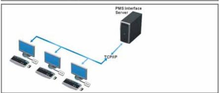
This is the most usual interface option with minimum configuration possible, Be-Tech software runs on the PMS server. Encoders connect to the PMS server PC or PMS terminal PC.
