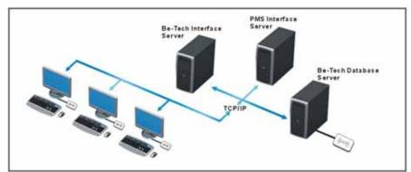
PMS terminal, additional Be-Tech server and PMS server share the Ethernet network. Encoders connect to the PMS terminal PC.
